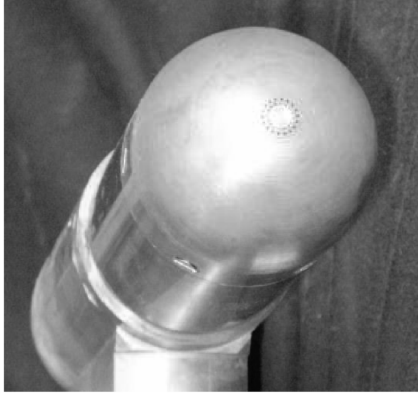
Fig. 1 Photograph of the enthalpy probe head.
